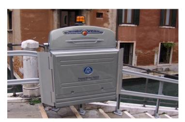
Figure 9: A Bridge Elevator
